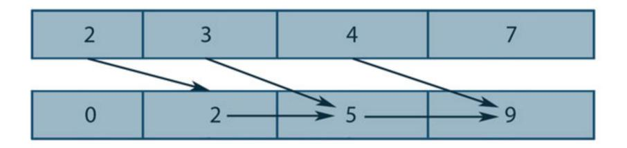
Each element i of the prefix sum array has the SUM of all elements which index is smaller than i
