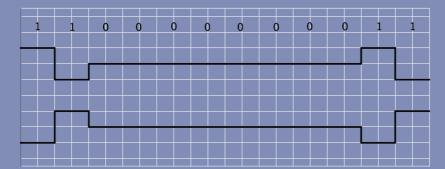
B8ZS (bipolar 8-zero substitution): Substitute eight '0' with:
