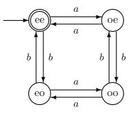
2.1(g2) When you consider the language of strings over  $\{a, b\}$  in which either the number of *a*'s or the number of *b*'s is odd (or both), you can take almost the same finite automaton. Only the accepting states and the nonaccepting states must be exchanged, because the language is the complement of the language from 2.1(g).
