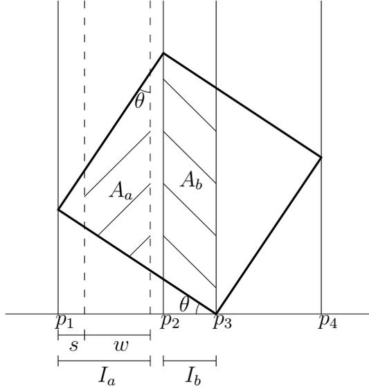
Figure 2.6: Projected mass calculation.
