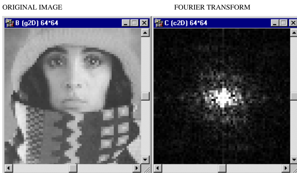
Figure 3-10 : The Fast Fourier Transform
