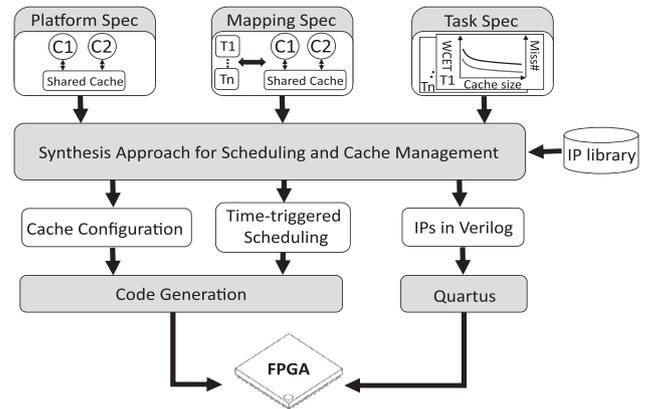
Fig. 4. System design framework.
