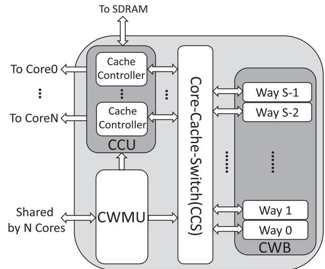
Fig. 7. Reconfigurable cache architecture.
