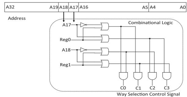
Fig. 2. Illustration of four-way set-associative reconfigurable cache architecture in [24].
