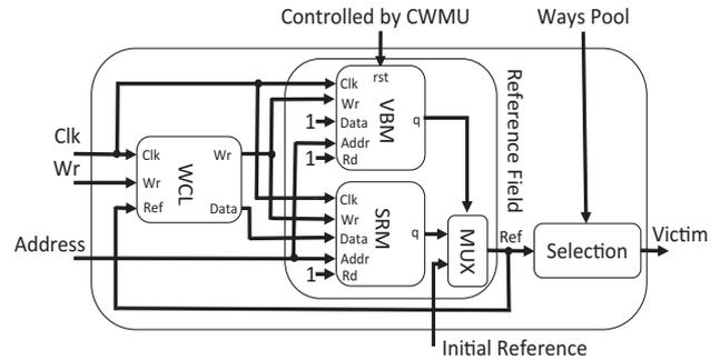
Fig. 10. Block reference field logic (BRFL).
