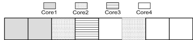
Fig. 3. Way-based cache partitioning.
