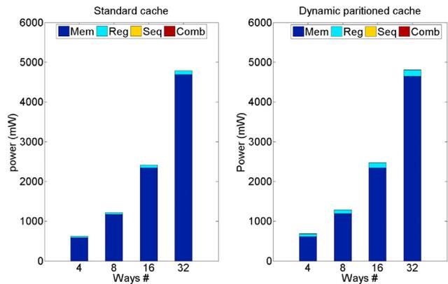
**Fig. 13.** Power consumption for dual-core caches with the varying cache way numbers.
