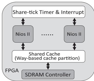
Fig. 5. System architecture.
