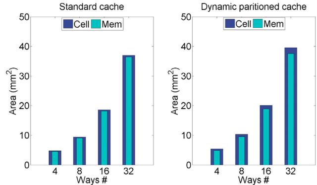
**Fig. 12.** Chip area for dual-core caches with the varying cache way numbers.
