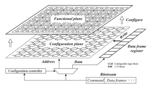
Fig. 1 Conceptual diagram of FPGA
