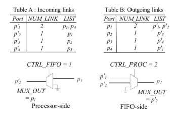
Fig. 4 Parameterised switch for MJPEG{4,5} topology in Fig. 3
