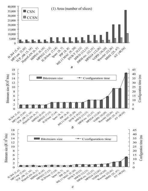
Fig. 11 Area and configuration overheads of CSN and CCSN in Virtex-II Pro xc2vp100
