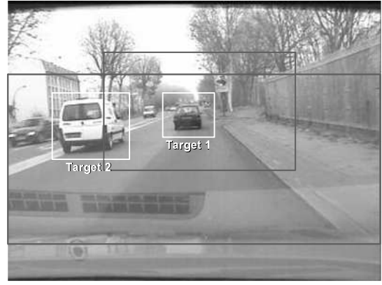
Fig. 2: LSOD applied on real data. The vehicles in front of the camera are detected and tracked. The dark rectangles depict the area of the image that is processed.
