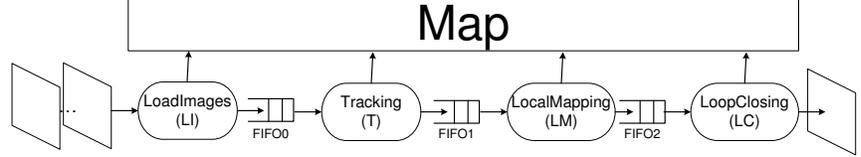
Fig. 2: KPN model of ORB-SLAM2
