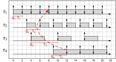
Fig. 2. The SPS of the CSDF graph  $G$  in Fig. 1 without considering the backward edge  $e_5$ . Up arrows are job releases and down arrows job deadlines.
