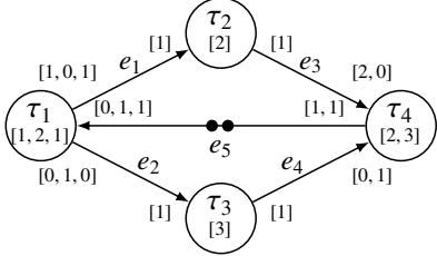
Fig. 1. A cyclic CSDF graph  $G$ . The backward edge  $e_5$  in  $G$  has 2 initial tokens that are represented with black dots.
