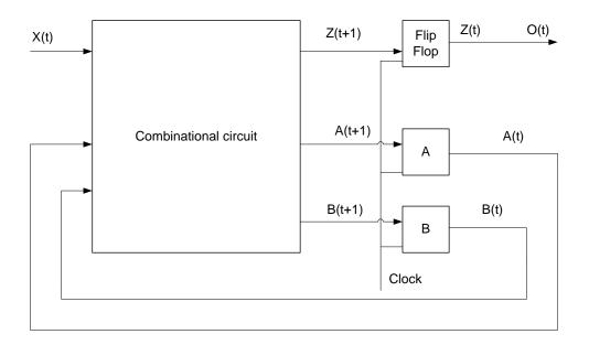
We get the following equations from our circuit (because of the Moore machine)  $A(t+1) = X(t)^{A}(t) + X(t)B(t)$   $B(t+1) = X(t)^{A}(t)^{Y}$   $Z(t+1) = X(t)A(t) + X(t)B(t)^{Y}$ O(t) = Z(t) Here is the combinational circuit block based on the equations.
