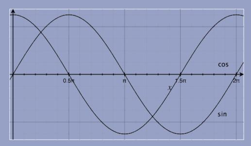
Sufficiently different in phase so that I(t) and Q(t) can be isolated.
