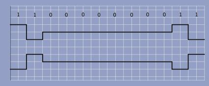
B8ZS (bipolar 8-zero substitution): Substitute eight '0' with:
