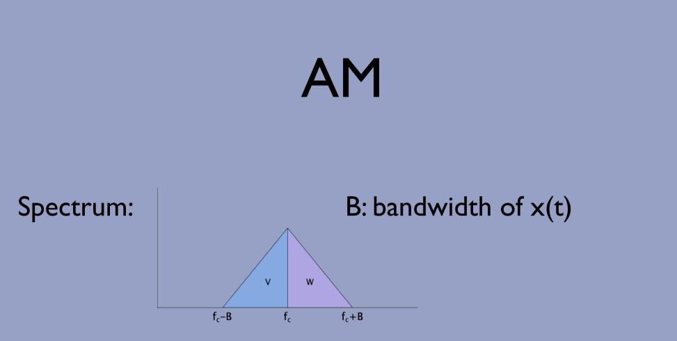
$V \equiv W$ , so all frequencies between f<sub>c</sub>-B and f<sub>c</sub> can be filtered away. Single Sided Band (SSB) instead of Double Sided Band Transmitter Carrier (DSBTC)
