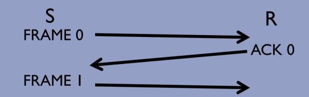
Transmission time per frame: t + 2a instead of t + a So if a (latency) is comparable to t (frame processing time), then 30% efficiency loss !!!!!!
