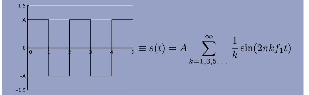
In addition to the time domain function s(t) there is also a frequency domain function: S(t), that gives the max amplitude per frequency. For the sum of the first three sines we have:
