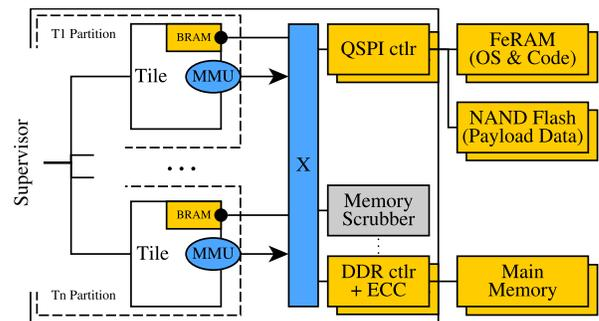
Fig. 2: The topology of our tiled MPSoC design. Each tile exists in its own reconfiguration partition, simplifying routing and clocking.
