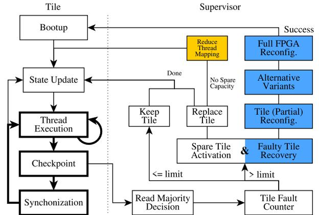
Fig. 1: Stage 1 (white) assures fault detection (bold) and fault coverage, Stage 2 (blue) and 3 (yellow) counter resource exhaustion.
