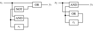
Each circuit has one input, output and register. For the first circuit, we have  $X_1 = \{x_1\}$ ,  $Y_1 = \{y_1\}$  and  $R_1 = \{r_1\}$ , while for the second we have  $X_2 = \{x_2\}$ , etc. To describe circuits formally, let  $\mathbb{B}$  be the set  $\mathbb{B} = \{0, 1\}$  of Boolean values. We define *valuations* for a given set U to be the set of functions from U into  $\mathbb{B}$ :
