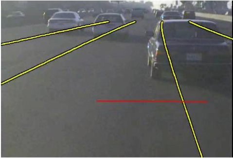
Fig. 16. Error due to occlusion of the road by a vehicle on the dusk dataset on road segment C. The red horizontal line shows the proximity of the occluding vehicle detected by the in-vehicle LASER RADAR sensors.
