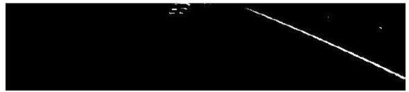
(c) Results from filter for a line tuned to the lane angle.
