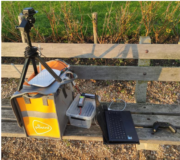
ZED-F9P Base Station
