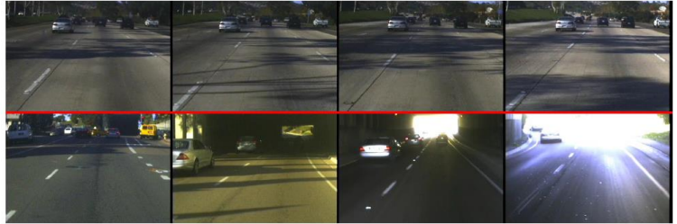
Fig. 17. Scenes from the special case scenarios of complex shadowing (top row) and tunnels (bottom row). These scenes highlight the extreme variability that can occur within short sections of road.
