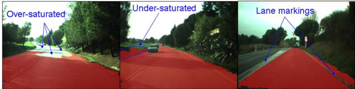
Fig. 13. Examples where our road-detection method currently fails.
