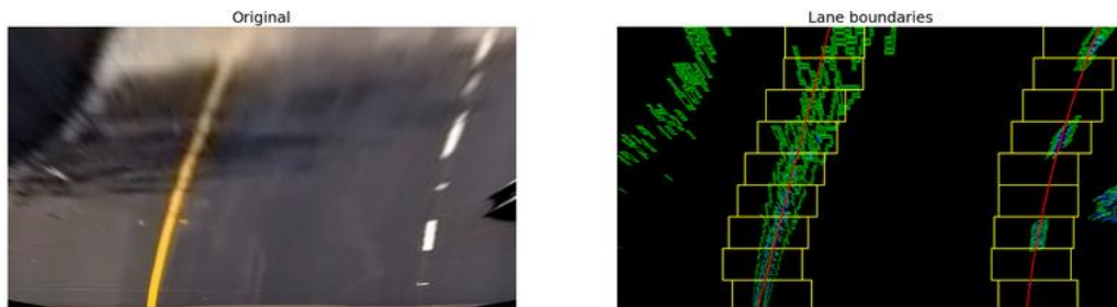
Boundary detection pipeline
