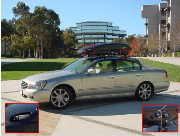
Fig. 11. The LISA-Q intelligent vehicle test bed. Inset are close up views of the front camera (left inset) used for detection and tracking and side camera (right inset) used for generating ground truth.
