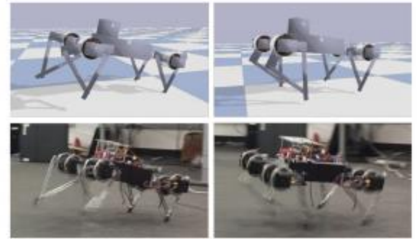
Fig. 1: The simulated and the real Minitaurs learned to gallop using deep reinforcement learning.
