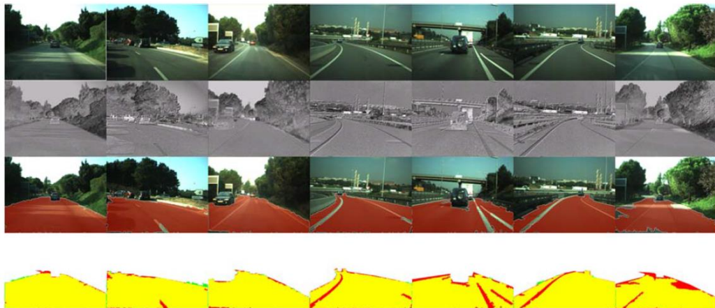
Fig. 11. Road-detection examples. (Top row) Original image. (Second row) Illuminant-invariant image. (Third row) Detected road. (Bottom row) Comparison against hand-segmented result. (Yellow) Correctly classified pixels. (Green) Falsely detected road pixels. (Red) False background pixels.
