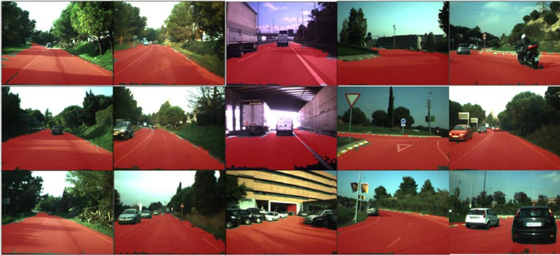
Fig. 12. Road-detection results. Example results include the following: (First column) Images from a sunny day with annoying shadows and traffic; (second column) images from a wet road without puddles with dim shadows and traffic; (third column) different scenarios; (fourth column) different road shapes; (last column) presence of other vehicles.
