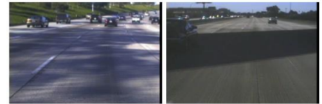
(e) Highly cluttered shadows from trees obscuring lane markings (f) Freeway overpass causing extreme lighting changes and reducing road marking contrast
