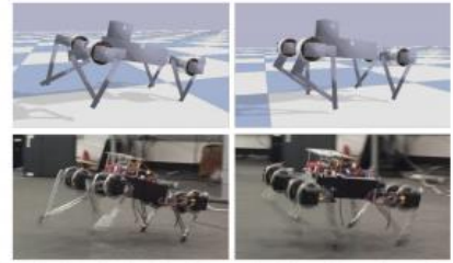
Fig. 1: The simulated and the real Minitaur learned to gallop using deep reinforcement learning.
