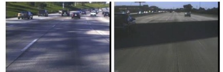
(e) Highly cluttered shadows from trees obscuring lane markings (f) Freeway overpass causing extreme lighting changes and reducing road marking contrast
