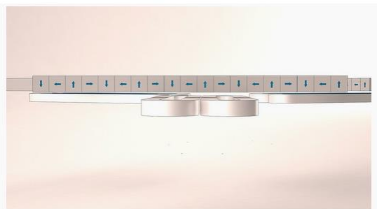
The Halbach arrangement of the magnets makes it possible, to minimize the energy required by the active coils in the stator for carrying the platform, to increase the load carrying capacity and to reduce thermal load
