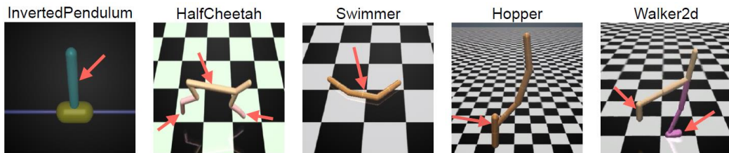
Figure 1. We evaluate RARL on a variety of OpenAI gym problems. The adversary learns to apply destabilizing forces on specific points (denoted by red arrows) on the system, encouraging the protagonist to learn a robust control policy. These policies also transfer better to new test environments, with different environmental conditions and where the adversary may or may not be present.
