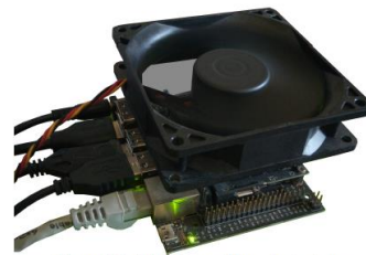
Figure 15: The Jetson Nano test setup
