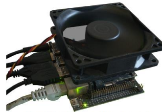
Figure 15: The Jetson Nano test setup
