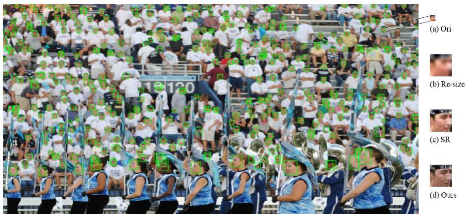
Figure1. The detection results of tiny faces in the wild. (a) is the original low-resolution blurry face, (b) is the result of re-sizing directly by a bi-linear kernel, (c) is the generated image by the super-resolution method, and our result (d) is learned by the super-resolution ( \times 4 upscaling) and refinement network simultaneously. Best viewed in color and zoomed in.
