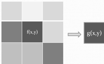
$$g(x, y) = \omega * f(x, y) = \sum_{dx=-a}^a \sum_{dy=-b}^b \omega(dx, dy) f(x + dx, y + dy)$$
