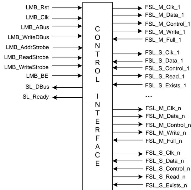
Figure 3.4: LMB FIFO controller interface.
