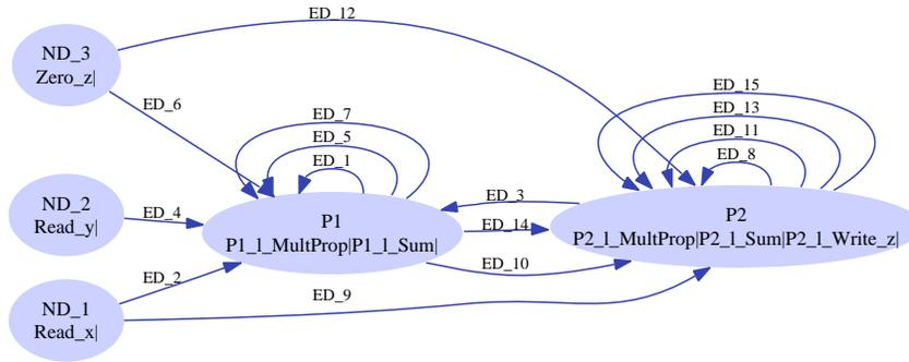
Figure 4.2: Unfolding factor = 2.
