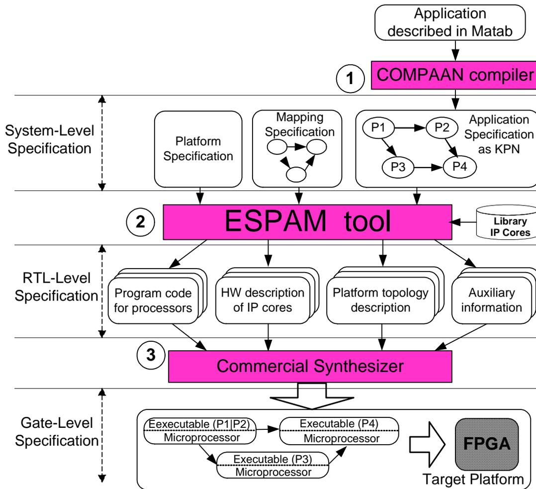
Figure 1.2: System design flow.
