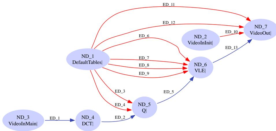
Figure 5.3: PRDG graph for the fully pipelined M-JPEG Application.
