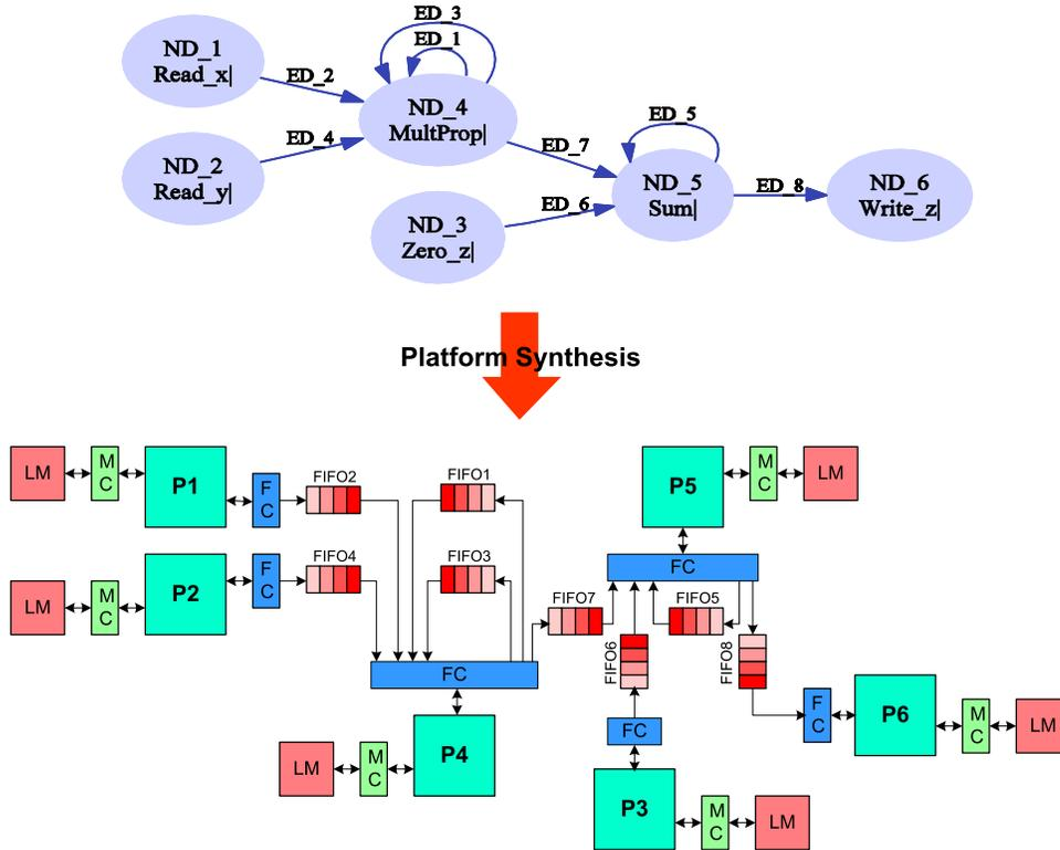
Figure 2.4: Synthesis of multiprocessor platform for KPN.
