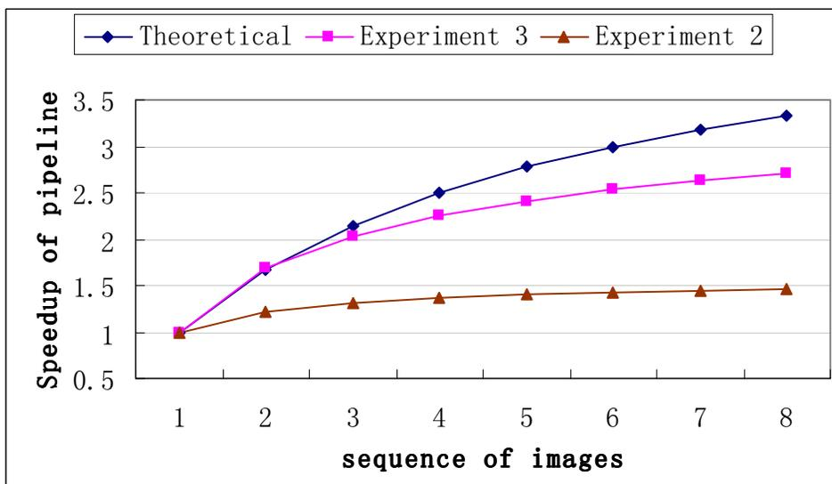
Figure 4.11: Speedup comparison of the theoretical value and actual value.
