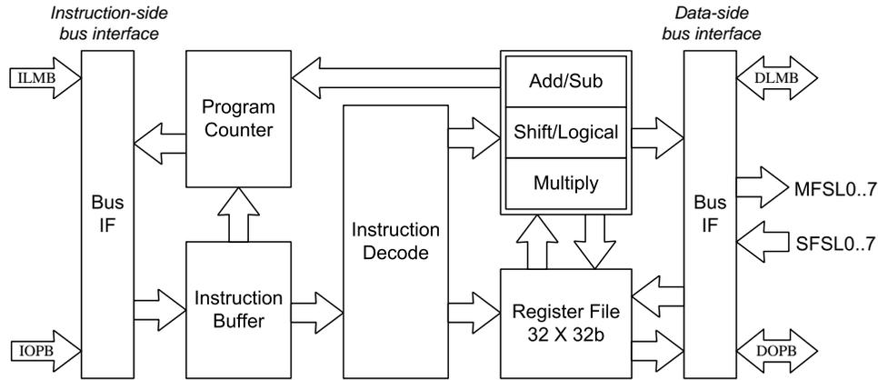
Figure 3.3: MicroBlaze core block diagram.
