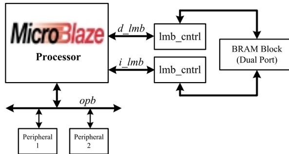
Figure 3.1: Simple MicroBlaze processor system.
