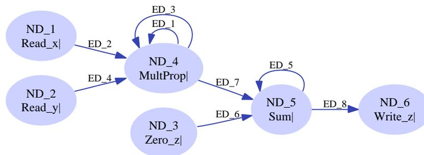
Figure 2.3: The KPN specification of the matrix multiplication.
