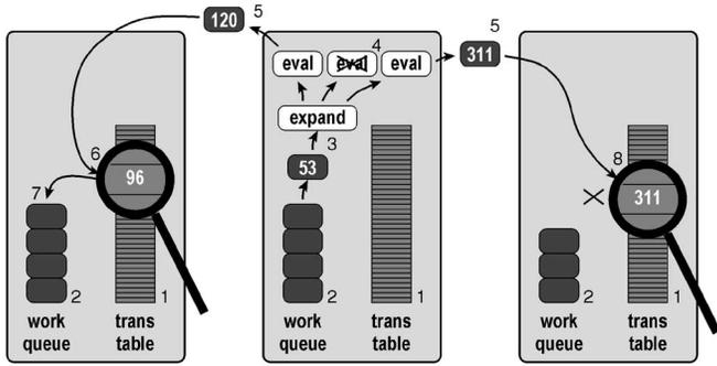
Fig. 3. Transposition-Driven Scheduling for IDA\*. Black numbers are referred to in the text.
