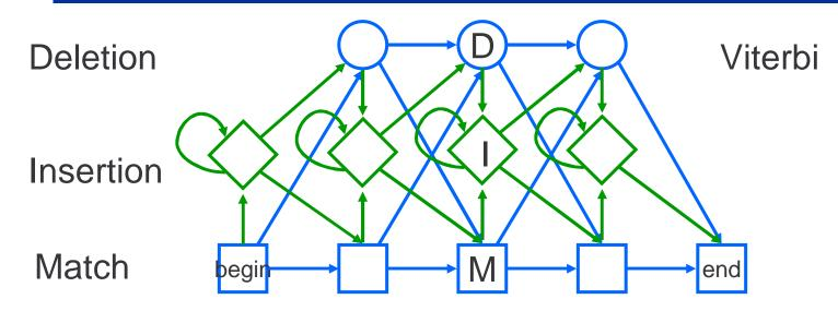
$$v_{j}^{M}(i) = e_{M_{j}}(x_{i}) \cdot \max_{Y=M,I,D} v_{j-1}^{Y}(i-1) t_{Y_{j-1}M_{j}}$$
