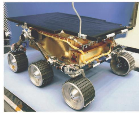
NASA's Mars Sojourner Rover (July 8, 1997) Microprocessor: 8-bit Intel 80C85 (produced 1977-1990)
