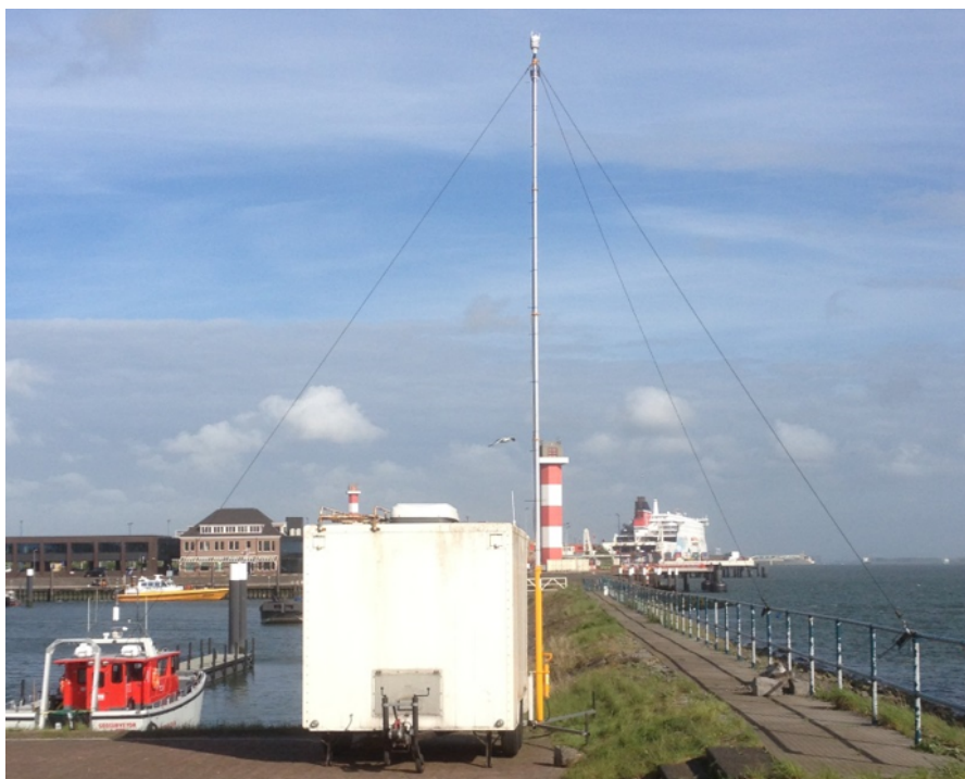
Figure 2.6: Sniffing set-up used by ILT and operated by TNO, which is located by Rotterdam. Taken with permission from [38].
