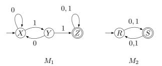
(a) Using the product construction, construct a finite automaton M from  $M_1$  and  $M_2$ , such that  $L(M) = L_2 \setminus L_1$ . Indicate M's initial state, set of accepting states and fill-in the following transition table.
