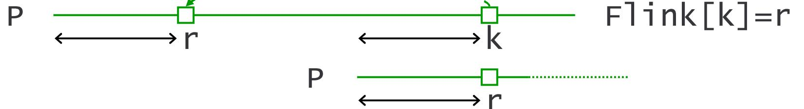
$$P_1 \dots P_{r-1} = P_{k-r+1} \dots P_{k-1} \text{ maximal } r < k$$
