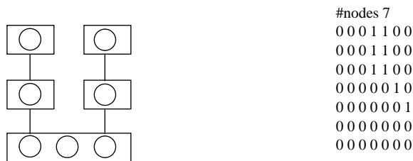
a) A modular network. b) The adjacency matrix of the network of fig. a
