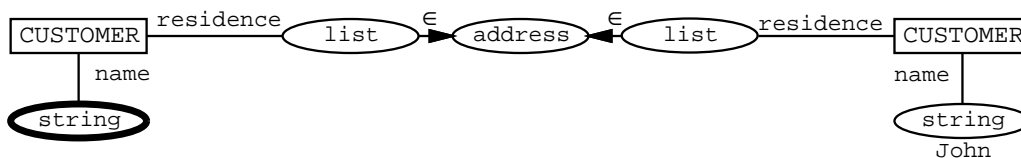
Figure 4.28: Names of customers sharing an address with John (HQL/EER version I, or GOQL/EER version)
