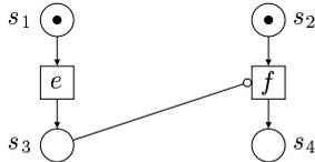
**Fig. 1.** An elementary net system with inhibitor arc.
