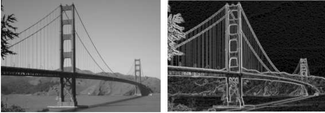
Figure 5.1: Original image (left) and the result of the Sobel operation applied to it (right).
