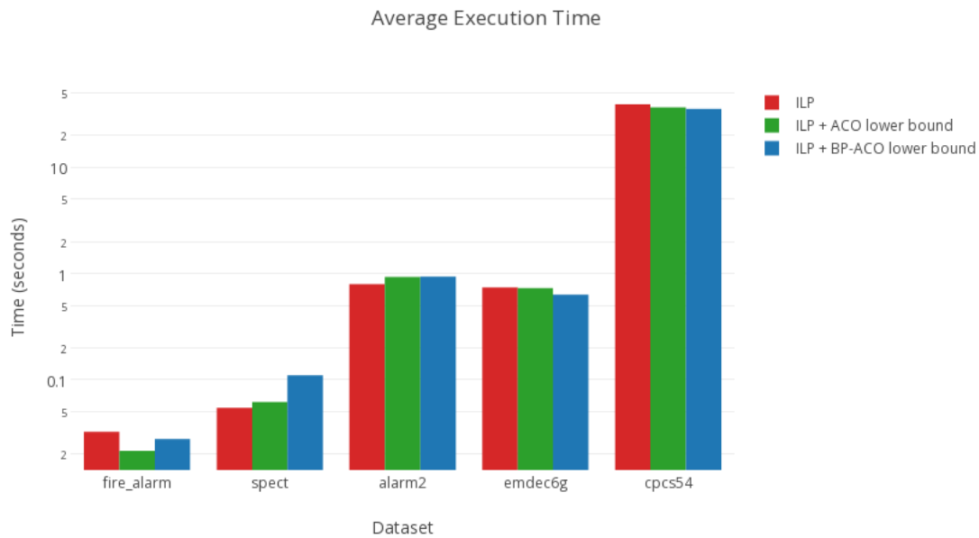
Figure 5.3: This bar plot displays the average execution time of the exact ILP solver on several datasets in three separate ways, using parameters \alpha = 1 , \beta = 1 , \rho = \frac{1}{10} , 2 iterations and 1 ant. The red bars show the execution time of just the ILP algorithm, the green bars show the execution time of the ILP algorithm using the solution from ACO as a lower bound and the blue bars show the execution time of the ILP algorithm using the solution from BP-ACO as a lower bound. The ACO and BP-ACO lower bounds do not lower the execution time of the ILP algorithm by much on the smaller datasets fire_alarm and emdec6g and even increase the execution time on spect and alarm2 . The biggest dataset ( cps54 ) however has an execution time decrease of 2.4 seconds using the ACO lower bound and a decrease of 3.5 seconds using the BP-ACO lower bound. The ILP algorithm without lower bound ran for 39 seconds on average.
