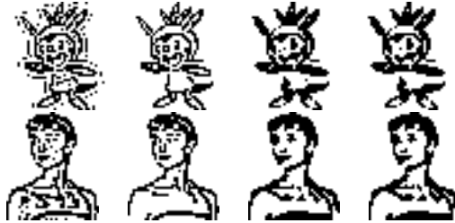
Figure 22: The first column depicts edge maps from applying fill30 on Laplacian 3\times 3 Block Kernel. The second column depicts edge maps from applying reduceWeakEdges on Laplacian 3\times 3 Block Kernel. The third column depicts edge maps from applying fill30 on Laplacian 9\times 9 Block Kernel. The last column depicts edge maps from applying reduceWeakEdges on Laplacian 9\times 9 Block Kernel.
